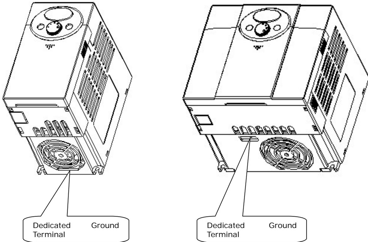
☞ Note : Remove front and bottom cover before starting grounding.
