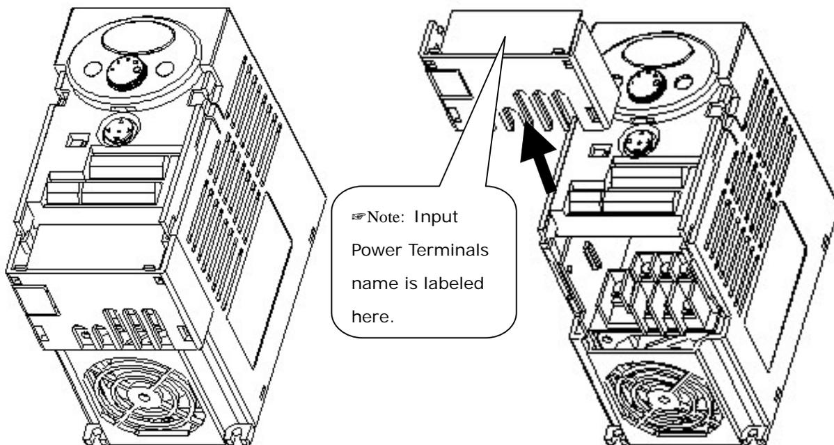
To access control terminals: after finishing power terminal wiring, reinstall the bottom cover and then start wiring control terminals.
