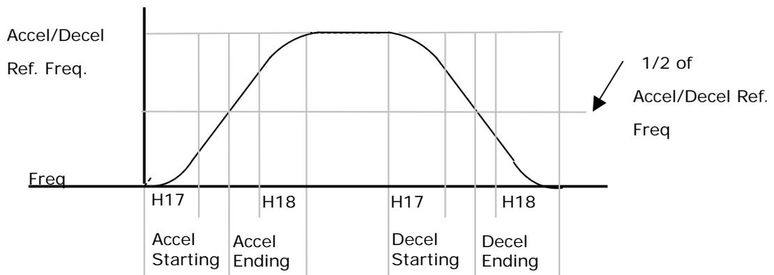
Note that setting Frequency Ref for Accel/decel (H70) is set to Max Freq and target freq is set below Max freq. the shape of S-curve may be distorted.
