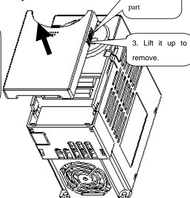
Removal for wiring input power and terminals: After removing the front cover, lift the bottom cover up to disconnect.
