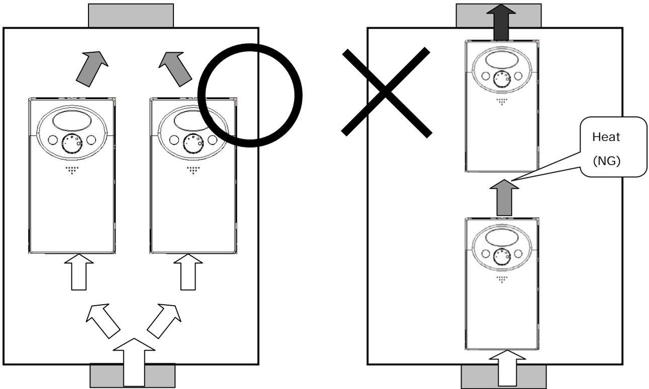
☞ Note : Take caution on proper heat ventillation when installing inverters and fan in a panel.
