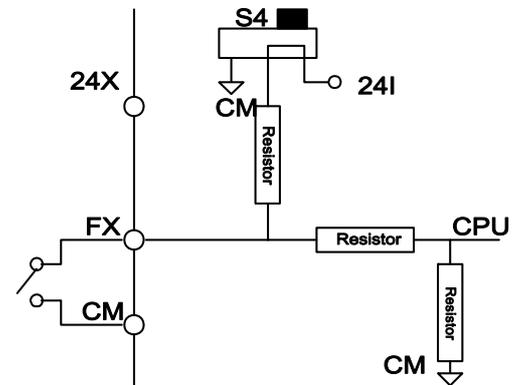
2. When using 24V external power supply [PNP]
