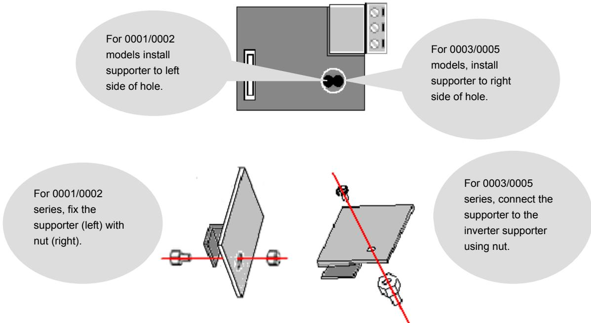
There are two holes on the option board for connection of option and inverter. Use left hole for models SINUS N 0001/0002 and right for models SINUS N 0003/0005 series.
