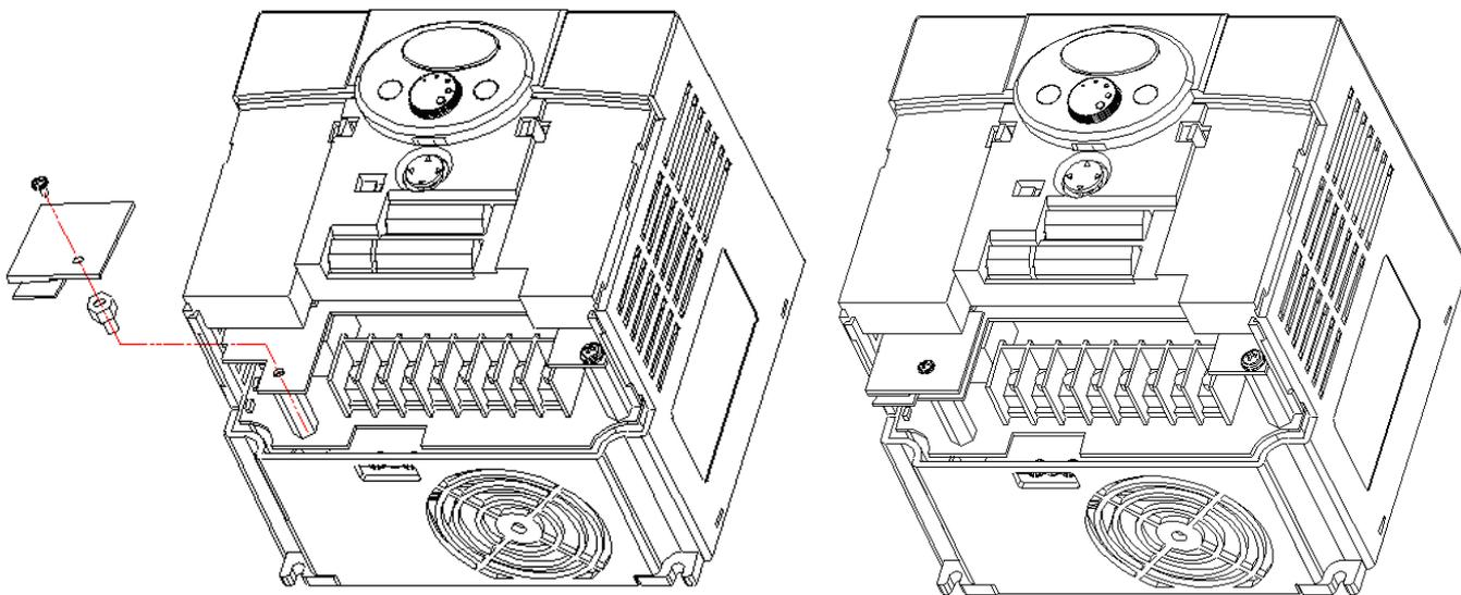
For models SINUS N 0003/0005 as shown above, loosen the bolt on the connector for Comm. Option and tighten it onto the supporter on the inverter case. Before fixing the option board, bottom cover plastic part for Comm. Option should be removed using knife or driver. The same method is used as 0001/0002 installation.
