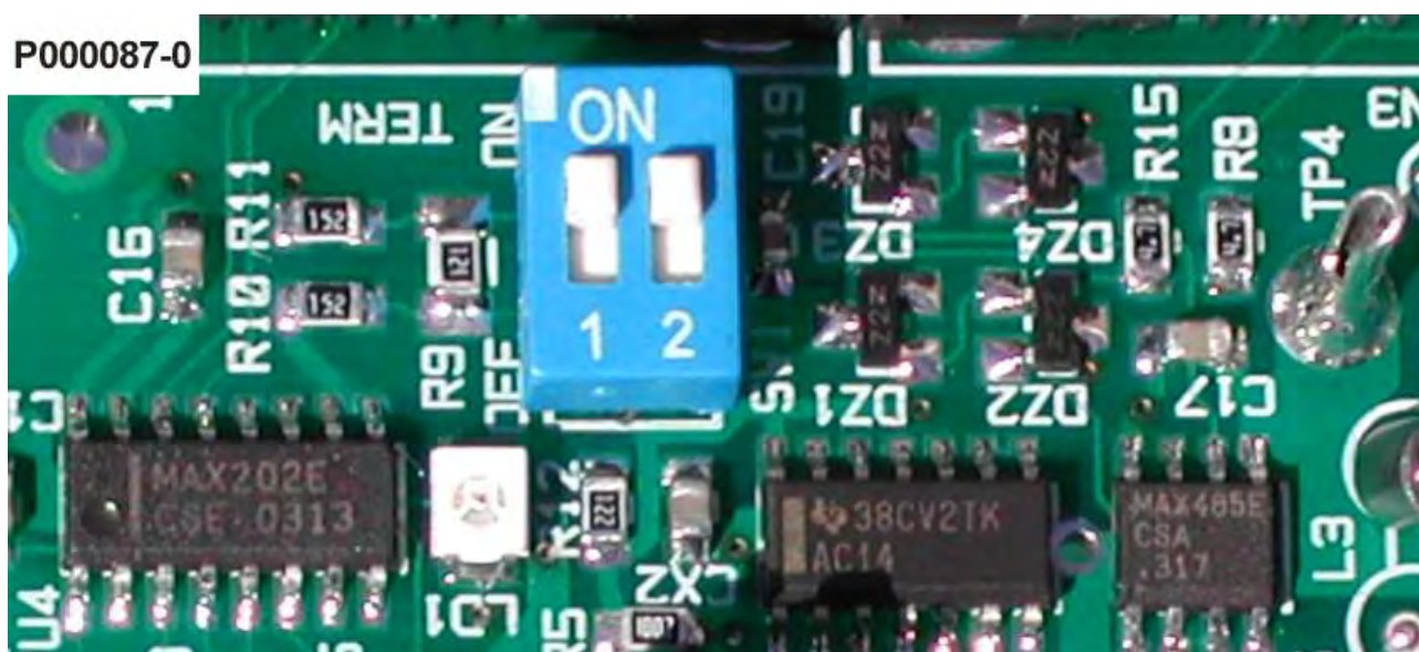
Figure 130: Configuration of terminator DIP-switch for line RS485
