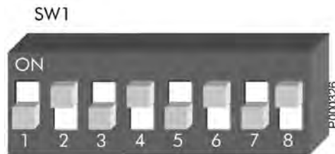
Figure 189: DIP-switch SW1 setting for five-channel mode
