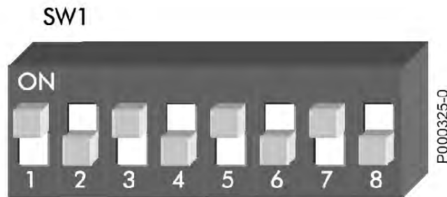
Figure 188: DIP-switch SW1 setting in three-channel mode
