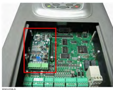
Figure 124: Encoder board fastened to its slot
