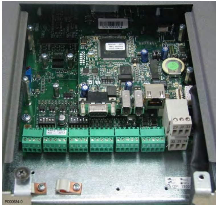
Figure 159: ES851 DataLogger fitted into slot B
