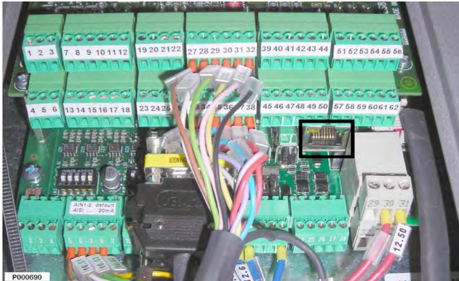
Figure 162: Location of the Ethernet port
