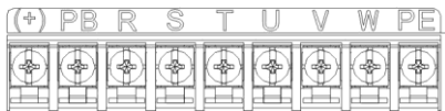
Figure 3-5 3PH terminals of main circuit (220V, \leq 0.75\text{kW} , and 380V, \leq 2.2\text{kW} )
